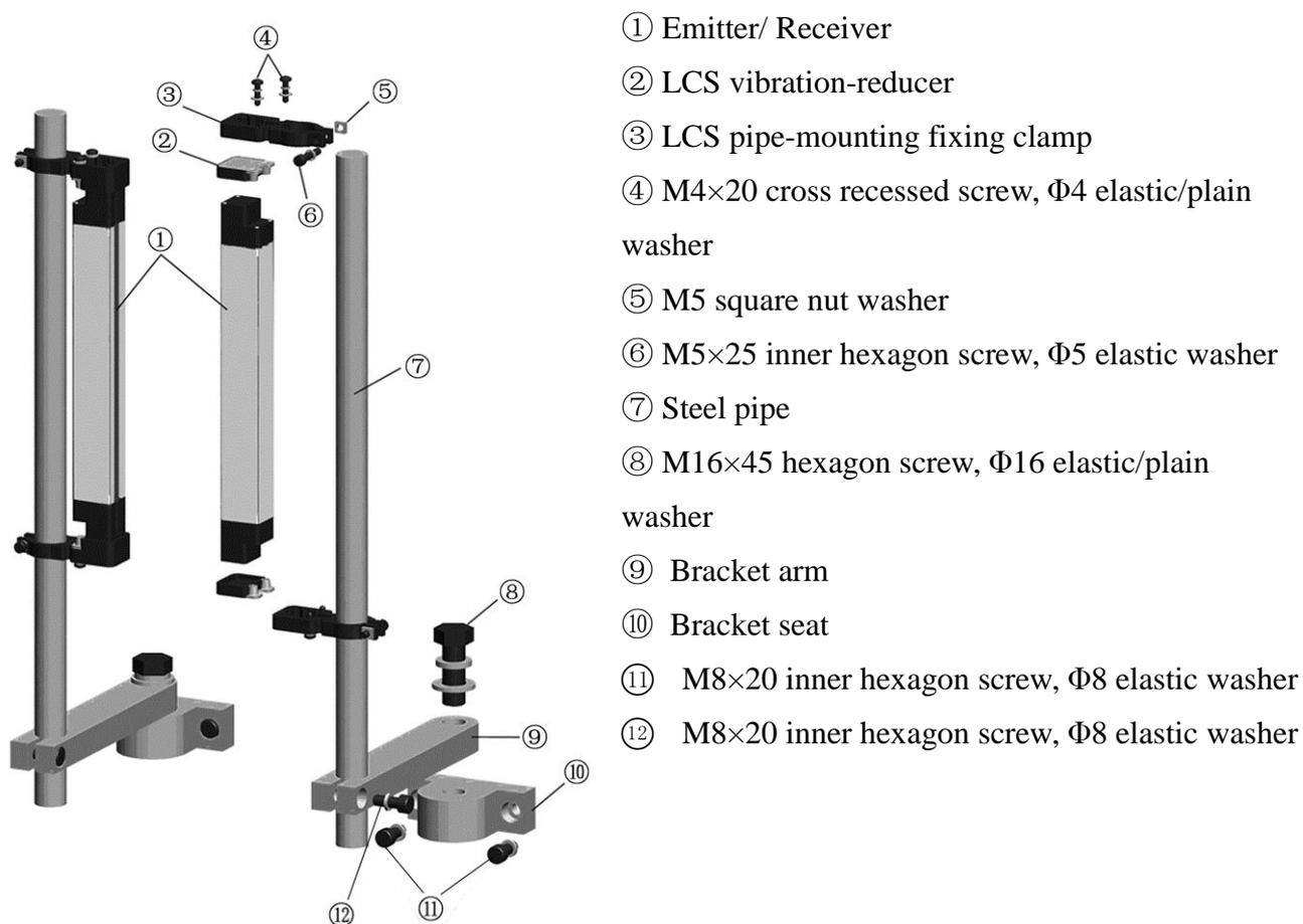
Fig.3.2.4 Pipe mounting installation (GZ)
