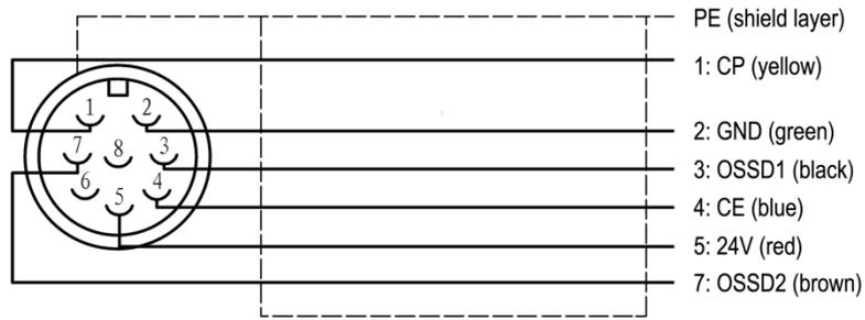
Fig.2.4.2 Signal definition of transmission cable
