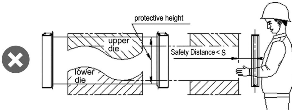
Fig.3.1.2 Incorrect installation position
