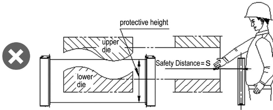
Fig.3.1.4 Incorrect installation position
