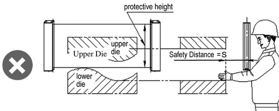
Fig.3.1.3 Incorrect installation position
