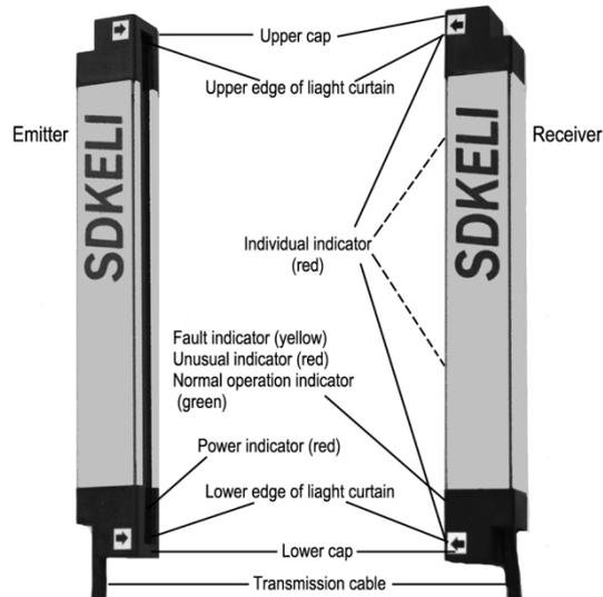
Fig.2.4.1 Schematic diagram of light curtain
