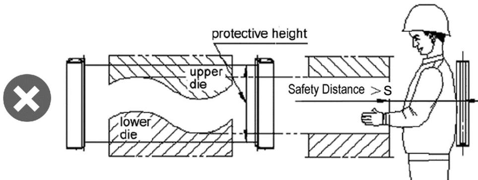
Fig.3.1.5 Incorrect installation position
