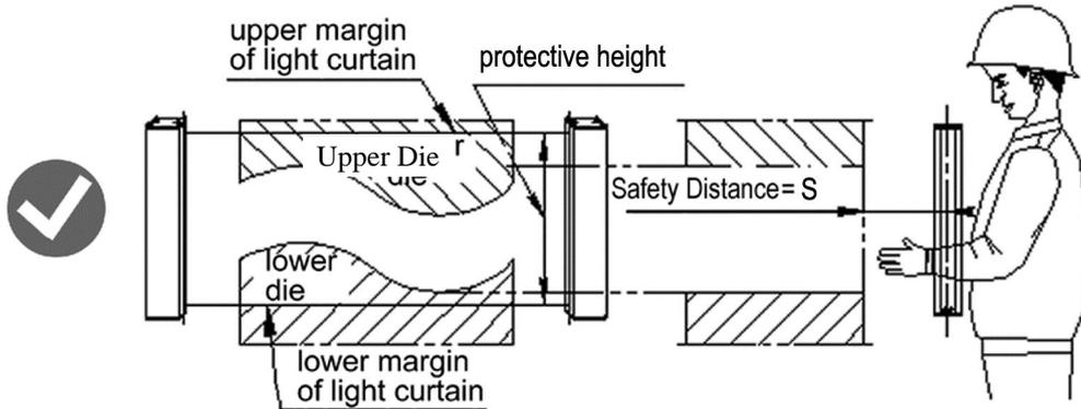
Fig.3.1.1 Correct installation position
