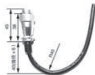
Dimensions of light curtain plug-in and maximum bending radius of cable
